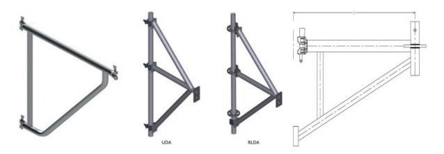
Side Triangle Bracket of Ringlock scaffolding is made of 48.3 mm with 3.2 mm wall thickness outside diameter galvanized tube.
